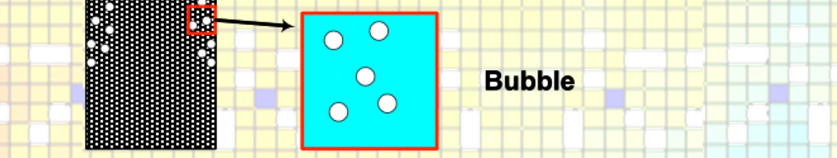
(Image Left) The two-phase boiling is based on an extended boiling framework which enables the simulation to model the local topology as bubbly flow, droplet flow or a sharp interface between steam and water. All of the boiling regimes that commonly occur in reactor systems can be reconstructed from these three local topologies.
